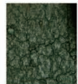
Laboratory reproduction of thermal fatigue cracks on metal mold
