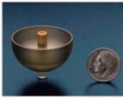
Hemispherical resonator made of fused silica ( Q = 25 \times 10^6 )
