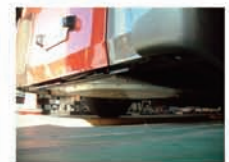
WPT coil for Electric Bus (30kW)
