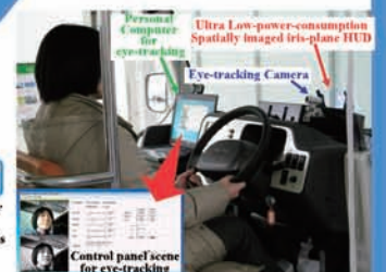
Fig. 7 Ultra Low-power-consumption Spatially imaged iris-plane HUD and Eye-tracking system mounted on Electric Vehicle Bus
