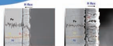
Evaluation of oxidation behavior for different penetration paths of hydrogen
