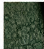
Laboratory reproduction of thermal fatigue cracks on metal mold
