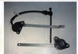
Rotary positioning sensor using the magnet (Automotive)
