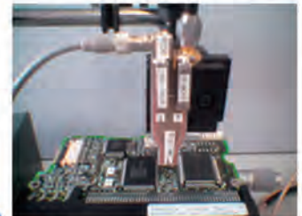
The measurement example by developed MI effect type magnetic probe
