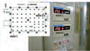
Seismometer in the Utility Floor 1 (B1F) observed largest peak ground acceleration of 250 Gal and seismic intensity of 6. (The largest peak ground acceleration was saturated at 250 Gal.)
