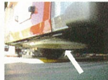
An actual 30kW Receiving Coil of EV Bus
