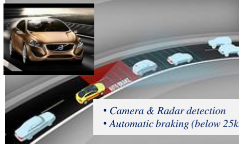
Volvo Pedestrian avoidance system (2011)
