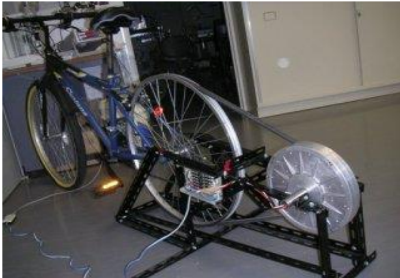
Fig. 1 Bicycle type human power electric generator : 200 ~600 W
