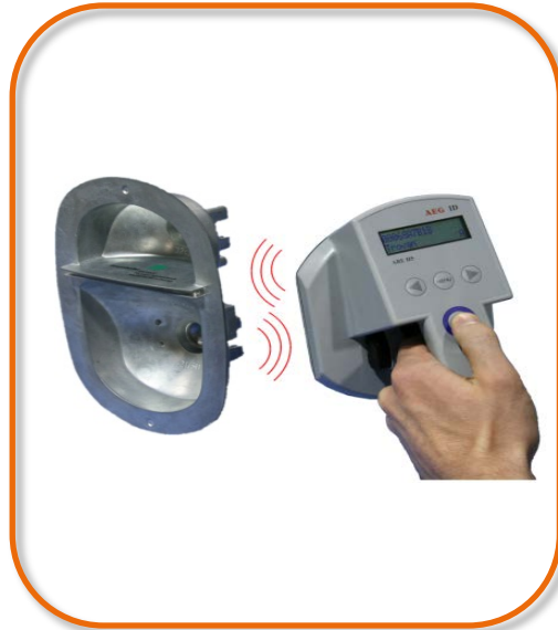
embedding of RFID transponder for part identification
