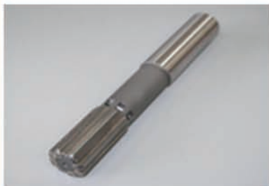
A prototype of burnishing reamer collaborating with companies
