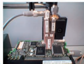
The measurement example by developed MI effect type magnetic probe
