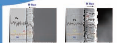
Evaluation of oxidation behavior for different penetration paths of hydrogen
