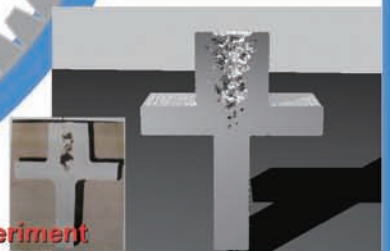
Result of interaction analysis of heat transfer and shrinkage using particle method
