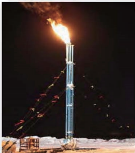
Natural gas released from gas hydrate is flared during cooperative DOE-ConocoPhillips-Japanese scientific production test on the Alaska North Slope, March 2012
