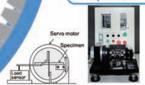
Load controlled plate bending fatigue test machine developed by Soyama Lab.
