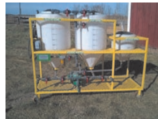
Fig. 1 Original bio-diesel reactor from Red Deer College
