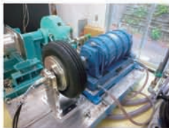
Motor Bench for In-Wheel Motor
