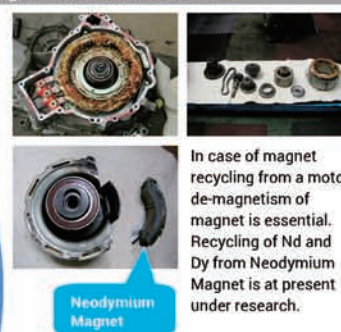
Fig. 4 Dismantling of Electric Motor in Electric Vehicle
