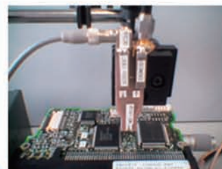
The measurement example by developed MI effect type magnetic probe
