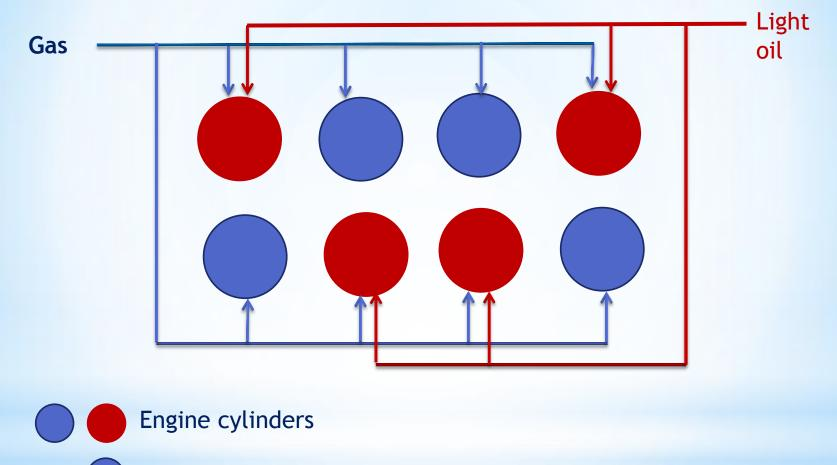
Ignited by spark. Used up to 1,000rpm or all rotation range.
