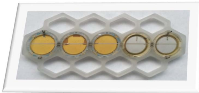
Actuator sections, SJA on the basis of MuCell® Technology
