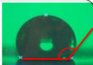
Fluoro-Wax Coated Surface \theta_c \sim 120^\circ
