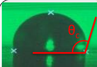
Paraffin Wax Coated Surface \theta_c \sim 100^\circ
