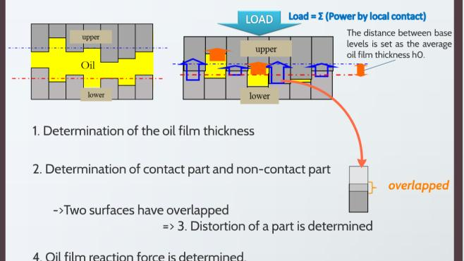
Determination of the oil film thickness (considering the elastic deformation)
