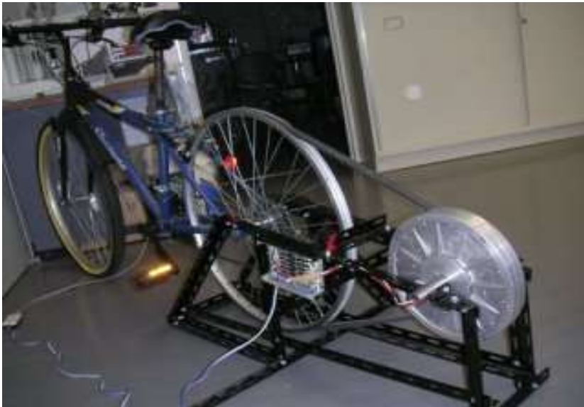
Fig. 1 Bicycle type human power electric generator : 200 ~600 W
